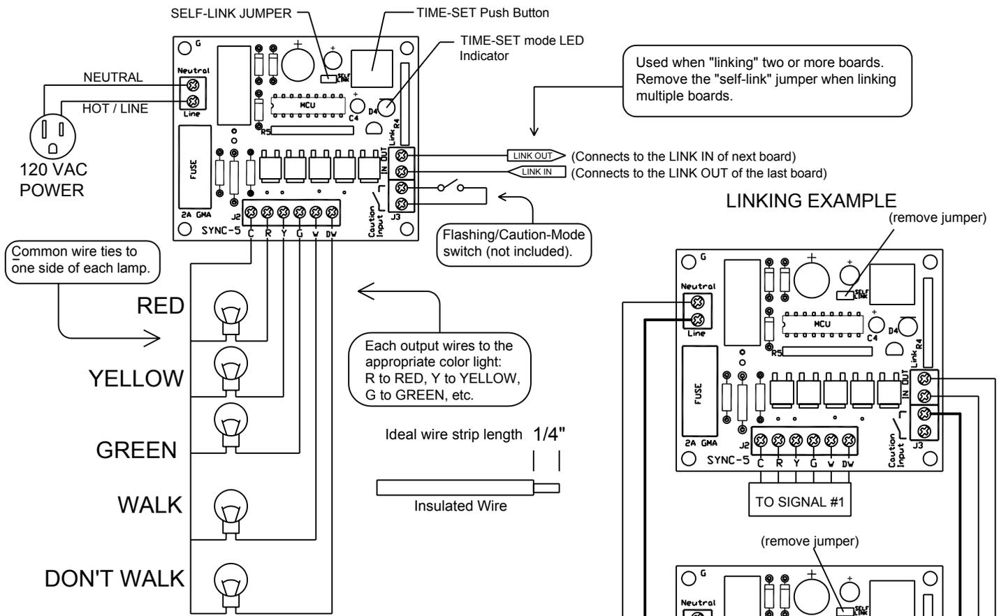
Used when "linking" two or more boards. Remove the "self-link" jumper when linking multiple boards.
